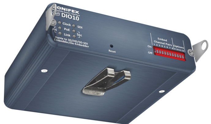
Fig 1-6: AVN-DIO Iso View Shown with AVN-DIOBT Brackets and Belt Clip Attached
